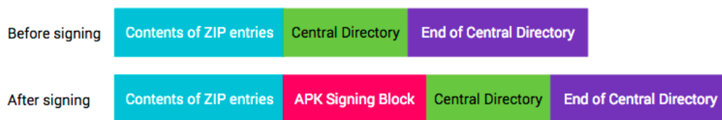
Figure 4.5: Signature location in an Android APK
